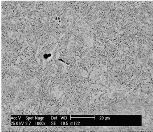
Fig. 5. SEM image of alloy 4 (NiAl+6Ga) corroded in 0.5 M NaOH solution.
